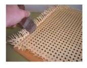
**3** Now the difficult part- but don't panic. Using a sharp Stanley knife, cut and trim off the excess rattan webbing no more than a couple of millimetres below the outer edge of the groove. Please try not to cut your wrist whilst doing this as it is very difficult to remove blood stains from the rattan webbing.
